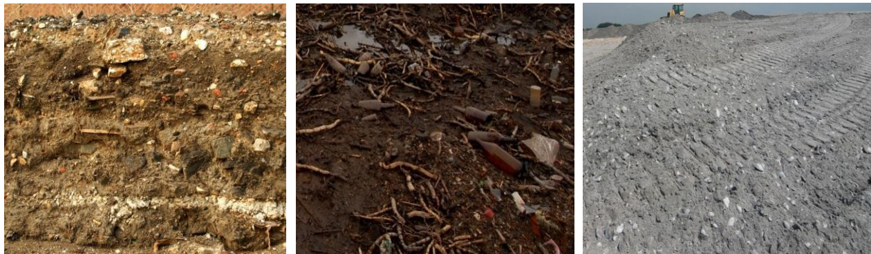
Figure 4. Examples of construction (left) and demolition fill, sanitation fill (middle), and dredge fill (right).
