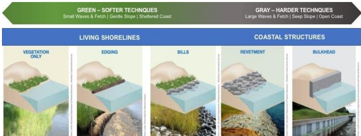
Figure 10. Green (nature-based) and gray (harder) shoreline protection methods for shoreline protection. Adapted from NOAA and USACE (2015) “Natural and Structural Measures for Shoreline Stabilization.”
