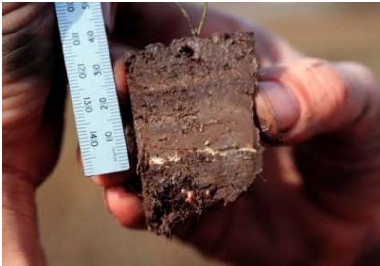
Figure 6. Measurement of accretion following placement of feldspar that acts as a marker horizon. Photo source: Don Cahoon, USGS, http://www.pwrc.usgs.gov/set/theory.html .
