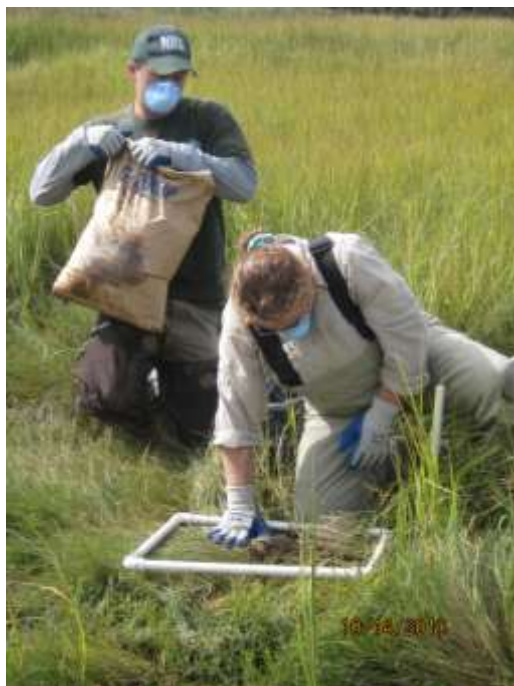
Figure 4: Photo shows the fourth pin being slid through the SET table to rest gently on the substrate surface for measurement. This is repeated four times at 90 degree angles for a total of 36 measurements and averaged to obtain a single SET data point (up to three times per year).
