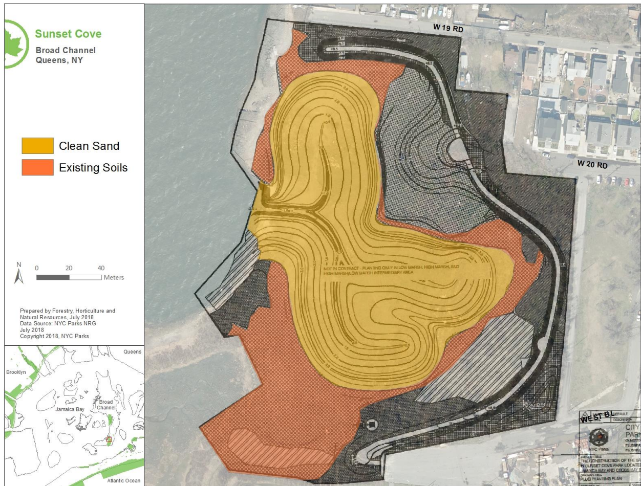
Figure 7. Sunset Cove restoration salt marsh substrate type map. Placed clean sand (gold) is where excavation will take place and the existing substrate (orange) will not be excavated.
